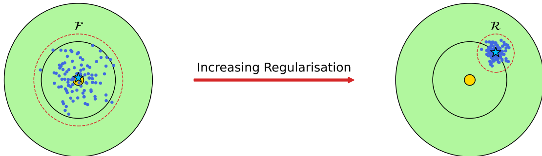
Figure 4.3: Visual demonstration of the effect of regularisation where the bullseye is the true value, the star is the cluster centroid, and each dot is a possible model output.
